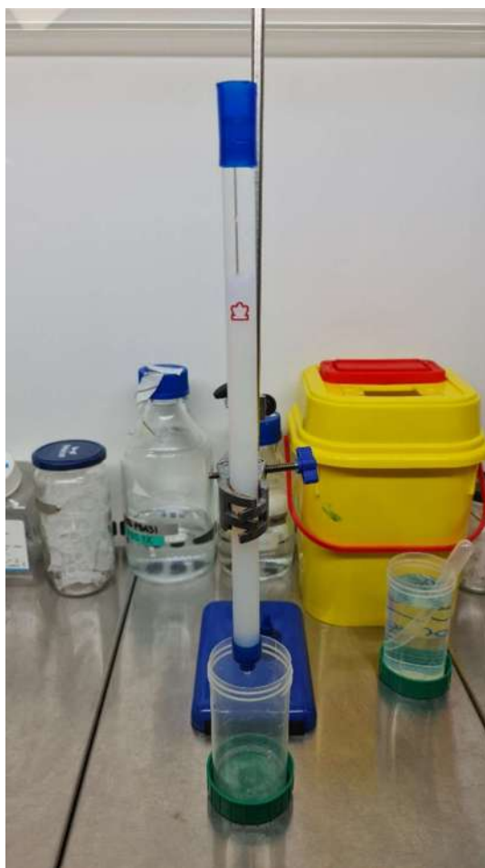
Figure 24. The SEC column used during the experiments.
