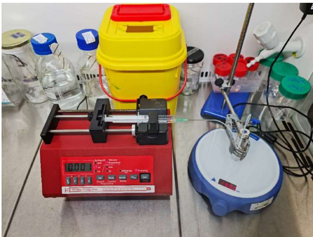
Figure 23. Set-up of solvent-switch method.
